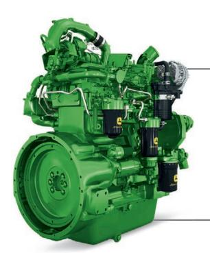
Our 4.5 L PSS engines (6R 110, 6R 120, 6R 130, 6R 140 and 6R 150) use a 2-stage turbocharging system in which the Wastegate turbocharger multiplies the pressure created by a fixed vane turbocharger. This sequential arrangement boosts power to achieve up to 131 kW (177 hp, max with IPM) in the 6R 150.
