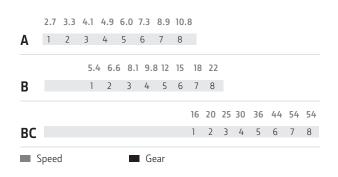
DirectDrive offers 11 gears between 4 and 12 km/h thus ensuring the optimum gear/rpm combination regardless of the situation.
