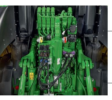
Depending on power demand, up to 30 additional kW (40 hp) for hydraulic applications get released with IPM.
