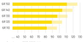
Rated power (ECE-R120), kWRated power with IPM (ECE-R120) at 2,100 rpm, kW (hp)
