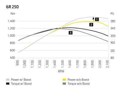
Intelligent Power Management (1) provides up to 30 additional kW (40 hp) for transport, hydraulic and PTO applications. Max. power (2) and max. torque (3) are achieved at 1,900 and 1,600 rpm respectively to ensure optimum response with low fuel consumption levels.
