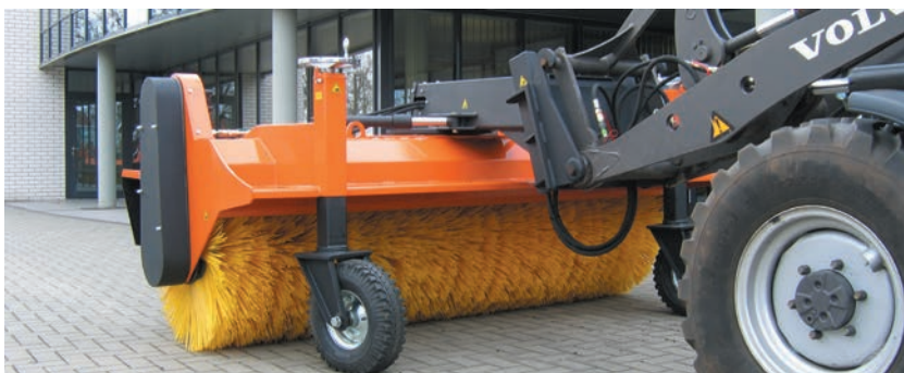
bema Jumbo on a wheel loader (quick change adaptor with roller levelling)
